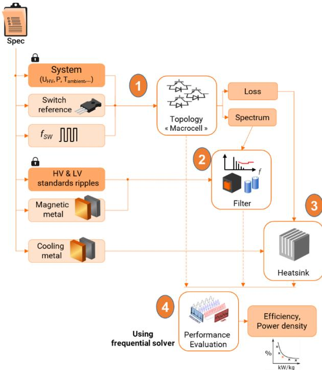
Fig. 10: Main steps of the design process
