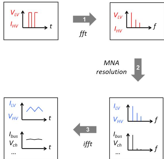
Fig. 3: Frequency resolution adapted to the commutation cell
