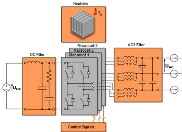
Fig. 9: Circuit of a multilevel three-phase inverter
