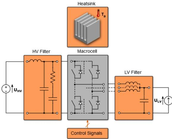
Fig. 8: Circuit of a multilevel non-isolated dc-dc converter
