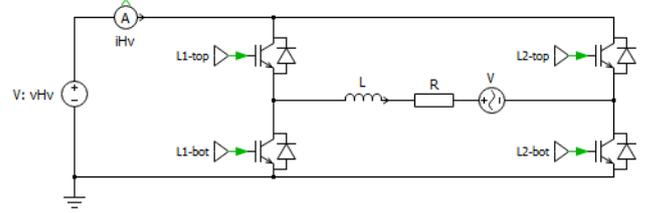
Fig. 5: Considered circuit composed of an inverter leg
